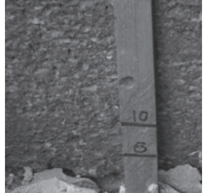
Photo 15: Soil spreading thickness and compacted thickness
