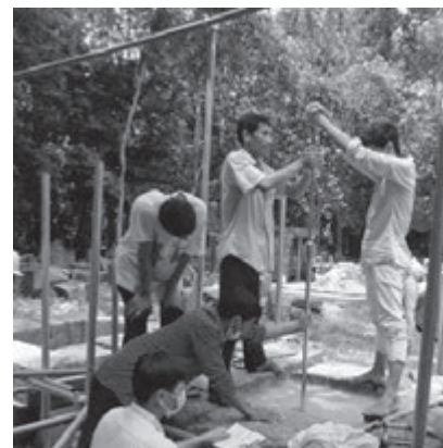
Photo 21: Quality inspection by a simple penetration test immediately after completion of the test foundation
