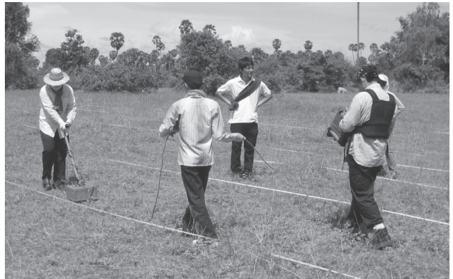
Fig 12. Geopenatratin Rader Survey in the school zone
