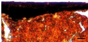
図7-2 P29-1-bの塗膜状破片断面
