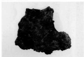
55-73 炉壁 (溶解炉・含鉄)
