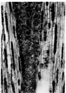
18b. コナラ節 (接線断面) bar:0.2mm
