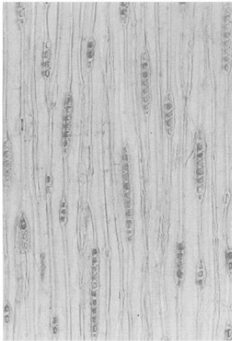
2b.ツガ属(接線断面) BKN-9 bar:0.2mm
