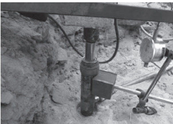
Photo 9: Water sprinkling around the load plate in a loading test
