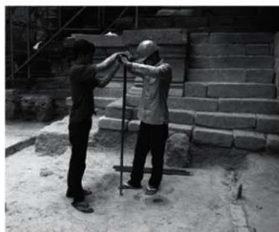
Fig. 69 (top left): Simple penetration test
