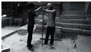
Fig. 4: Boring test using a hand auger
