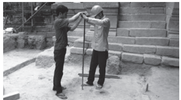
Fig. 4: Boring test using a hand auger
